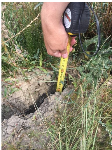
Figure 7 - Measurement of depth of shrinkage crack in embankment. (Photo Credit: Phil Welton)
